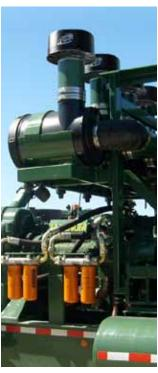
If dust, grit and dirt are a part of your daily operation, don't make your air cleaners do the job alone. Pre-cleaning the air entering the intake port can dramatically improve the life of air cleaners, and help avoid costly engine failure.
